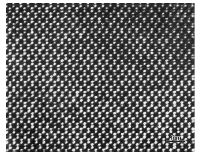
Fig. 1.12 Silicon atoms seen in a high-resolution transmission electron microscope (photograph courtesy of Jeol). Each spot can be identified with a single atom (although such an identification is not always possible).
